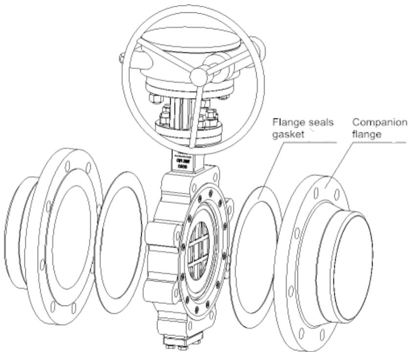
2.10 Use the correct size counter flanges, gaskets and fasteners, these parts should be suitable for the operating conditions. Flanges bolts should be tightened, using a tool to evenly load bolts.
